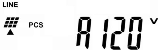
6.1.4 After 5 seconds, if the DC soft start of the inverter is successful, the LCD display will illustrate drawing D. The Green LED still flashes flickeringly.
